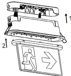
5 - Click the body back into the first fix section, ensuring the the connector(s) from the mains/DALI terminal blocks have been connected to the gear tray. Click the legend to the body ensuring it is the correct way round and observing the position of the charge LED.
