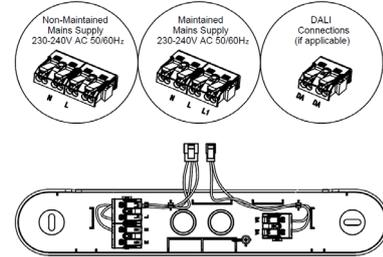
2 - Fit mains supply cables to the terminals as shown. Either maintained or non-maintained operation. Connect DALI cables if required. (DALI versions only).
