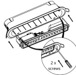
4 - Fit the gear tray back into the body, tightening the screws as shown.
