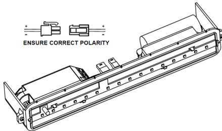
3 - Once mains supply is present, connect the battery cable connector together.
